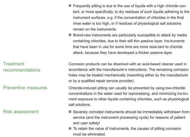
Corrosion holes can pose a hygienic hazard and may lead to stress corrosion cracking as well.
