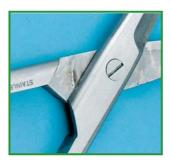
Fretting corrosion due to inadequate lubrication
