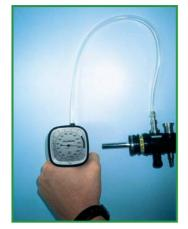
Manual leakage test on flexible endoscope
